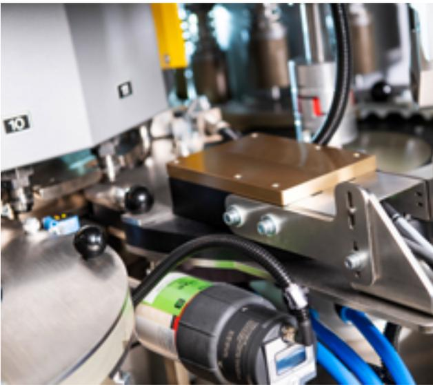
The TEM gives flexibility in the process sequence thanks to its modular design for slitting/folding or folding /slitting of the tamper-evident band. It also allows a large variety of cap dimensions, including sport caps.
