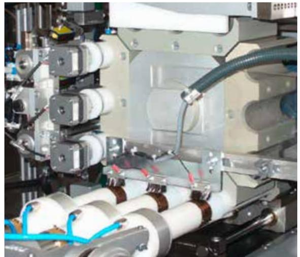
Fig. 2: Body orientation unit
