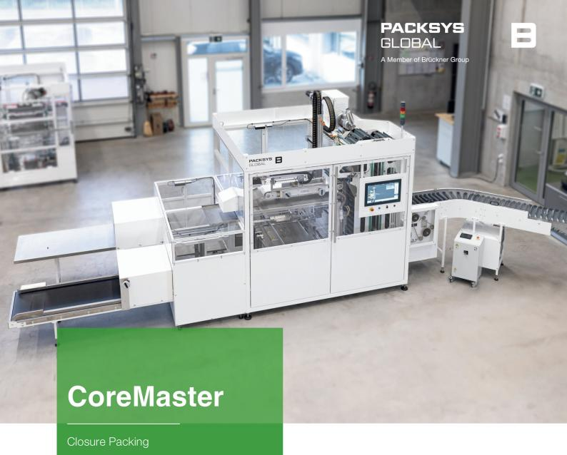
The CoreMaster closure packing machine packs beverage closures and is often connected to upstream machines. Both aluminium and plastic closures can be run at a speed of up to 165 closures per minute. The machine has its own control system, including the electrical cabinet, and is therefore autonomous.
