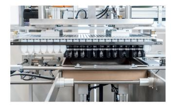
We offer synchronized transfer to the upstream machine, which is done by a servo motor in combination with an encoder or direct electronic input. Packing densities can be increased by 20% for 44mm high caps and 50% for 60mm high caps by regular packing patterns.
